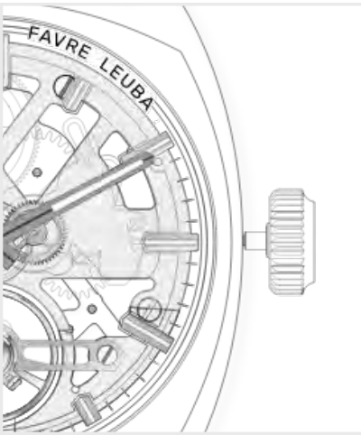
Position 1: Winding the Watch Unscrew the crown by turning it anticlockwise. After unscrewing, turn the crown clockwise to wind the watch
