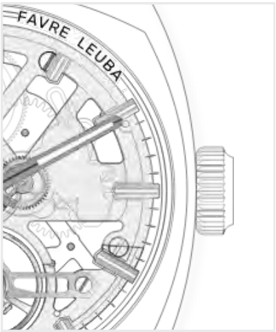
Position 0: Normal Position Crown closed
